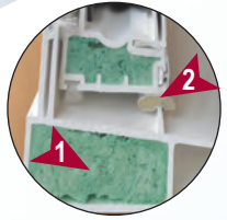
1) OPTIONAL Comfort-Foam™ insulated sash and frame extrusions improve thermal efficiency and reduce outside noise. 2) Our Q-Lon® compression gasket system adds barriers and diversions for exceptional water resistance.
