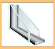
Stainless Steel Spacer Warm-edge stainless steel spacer system features a flexible, U-shaped design that reduces the surface area and mass of the spacer to allow expansion and contraction to improve seal life and reduce condensation. This system resists spacer movement and sealant failure and is 10° warmer than aluminum and 5° warmer than tin.
